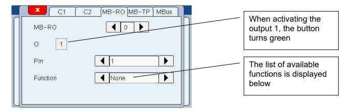
The MB-RO allows to manage the ACS-PNE-004 regulator to save air when measuring by air gage.
