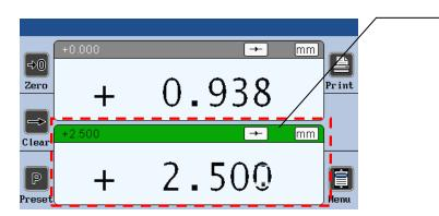
The lateral button have an effect only on the active characteristic
