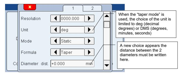
The half taper formula, will give the value of half an angle of a taper
