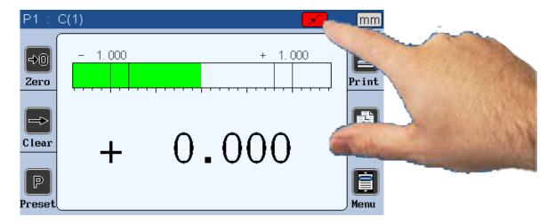
To change the measuring mode, press on the icon as shown on the above picture.
