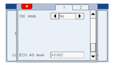
Thus the MB-RO modules "control" the air pressure of the preparation either in standard mode (measurement) or economy (no measurement, or action). And the indication of a wake-up threshold switches the air flow to standard mode, when for example the operator places a part back on the gage.
