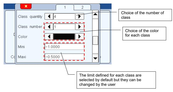
The class has an important utility, because it allows the user to sort the parts according to their position in the tolerance interval. The top bar of the display, which is normally blue is grey on the picture bellow, because grey is the color which was defined for this interval of measurement.
