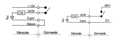
Command example: with internal supply (not isolated) and with an external supply (isolated).
