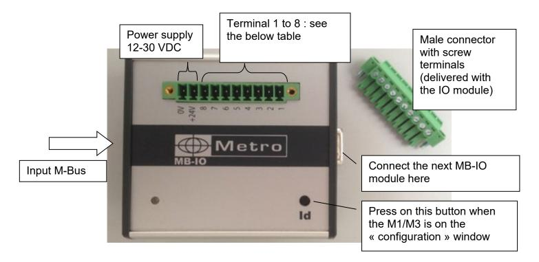
After adding the MB-IO module according to the process described in chapter 7.3.2, the configuration of the channels is done by clicking on the MB-IO tab
