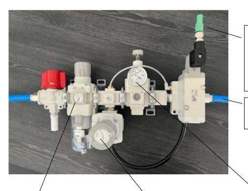
Controllable solenoid valve to regulate the air in standard or economy mode, connected with the M12 cable ref 45186
