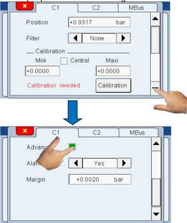
In measuring mode, if the input pressure has changed over the limit, a popup windows appear informing the operator, and asking the recalibrate, or check the air network.
