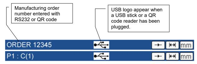
Note: When either a characteristic name or a manufacturing order name has been entered, only 1 information appear on the blue bar. However, the information display can be changed by touching the area:
