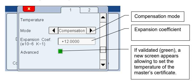
When the « compensation mode » is activated, it is requested to enter the expansion coefficient. As an information, on the below table you can see the coefficients of the main materials (source Wikipedia):
