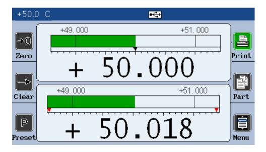
The « compensated characteristic », stayed at 50.000mm thanks to the compensation. (50.000mm is the dimension of the part at 20°C)
