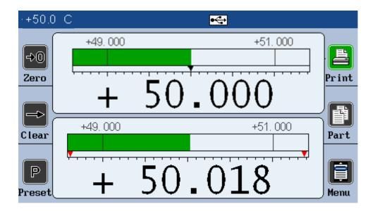
The » compensated characteristic », stays at 50mm, thanks to the master compensation during the calibration phase.
