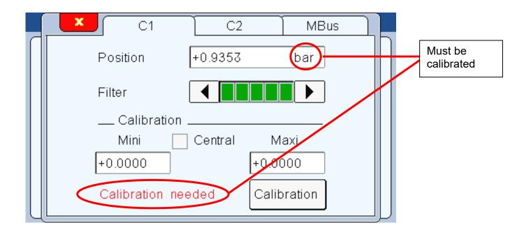
The air gage probes cannot be used without a special calibration. This calibration requires at least 2 master sample of the size of the tolerance limit for the part to measure.
