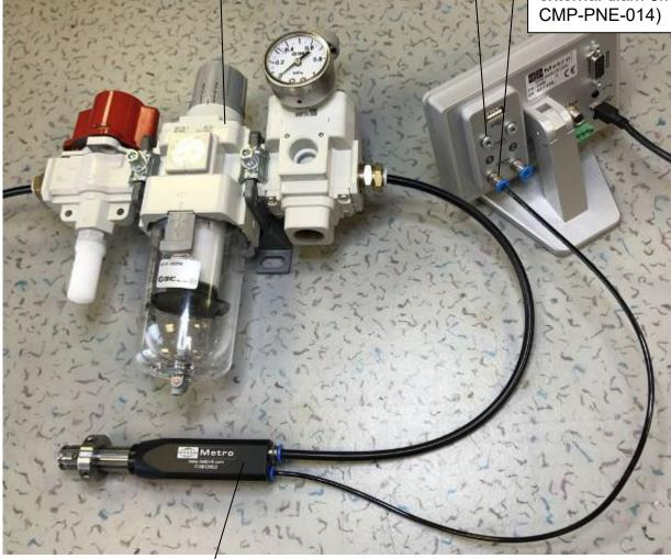
Air gage with by-pass nozzle (integrated restrictor)
