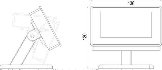
The M3 is fitted with 4 thread M5 allowing to attach it. To access to these threads, it is necessary to remove the 4 antiskid plastic parts.
