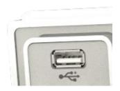
This connector allows to connect USB sticks and USB bar code readers (see chapter 12). It is possible to connect both at the same time using a USB hub.
