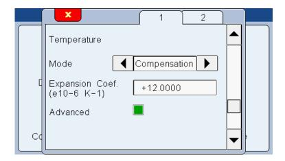
Then we tick the advanced mode to enter the reference temperature of the master, given by the certificate,
