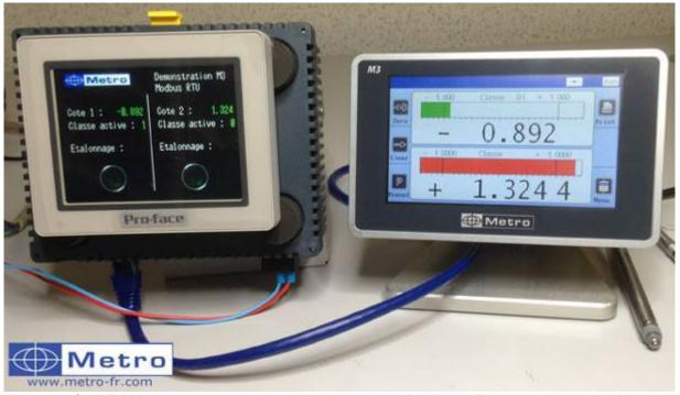
Example of a RTU Modbus communication with an automate Pro-Face. This example can be download from our website <a href="https://www.metro-fr.com">www.metro-fr.com</a>
