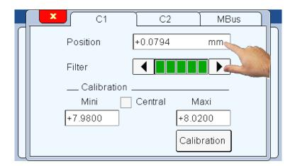
After calibration is it possible to check the pressure. For this you need to click on the unit "mm", the unit will then become BAR for few seconds.
