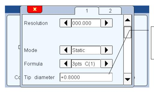
The size (diameter) of the tip must be written here in order to calculate correctly the diameters of the part
