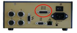
The external M-bus module has the same pinout (SUBD-15) than the relay board of the Monocote display, so there is no need to change the wiring of the existing installation.
