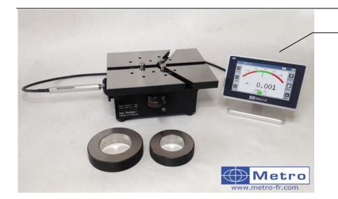
On this table 3 points, 2 points are fixes and the third one moves to constrain the part and measure its diameter
