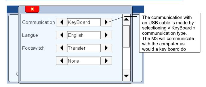
If you select the "Keyboard/USB" communication, the M3 will be detected has a keyboard when connected to a computer, without installing a specific driver or software.
