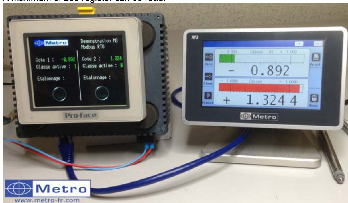
Example of a RTU Modbus communication with an automate Pro-Face. This example can be download from our website www.metro-fr.com
