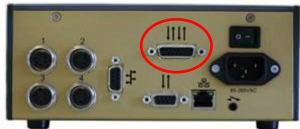
The external M-bus module has the same pinout (SUBD-15) than the relay board of the Monocote display, so there is no need to change the wiring of the existing installation.
