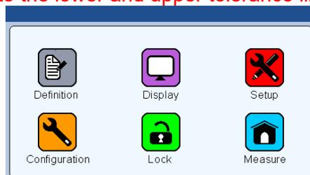
A – From the « SETUP » icon, write the master values according to your calibration certificate. The display need 2 masters MIN and MAX to be used.
