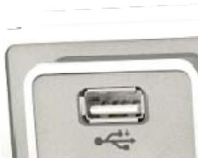
This connector allows to connect USB sticks and USB bar code readers (see chapter 12). It is possible to connect both at the same time using a USB hub.
