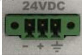
Using this power supply instead of the mini-USB will deactivate the ON-OFF switch. Therefore, when the M3 is powered, it will start automatically.
